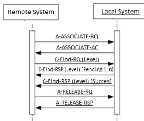
Figure 7: Data Flow Diagram – FIND as SCP
