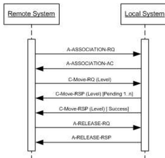
Figure 8: Data Flow Diagram – MOVE as SCP
